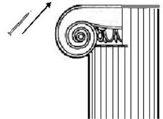
3. Repeat for the second half of the capital. Adjust as necessary to minimize any gaps at the seams.
