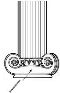
3. Place the assembled column on its side, then slide the base on the column shaft. Ensure the base aligns with the capital (do not secure).
