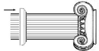
4. Set column in place and plumb with a level. Attach the capital to the upper structure by inserting the appropriate screws, thru pre-drilled holes in the ceiling end of the capital.
