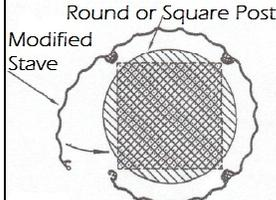
*Note: The stave with the modified lip has a portion of the inter-locking lip removed.*
