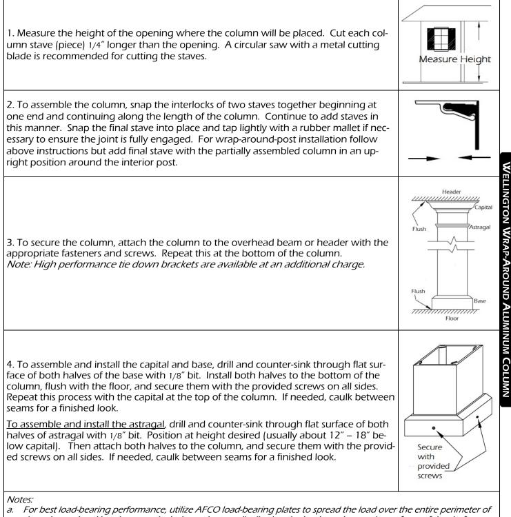
the column. Load-bearing capacity is dependent on distributing the load evenly over the surfaces of the shaft.
